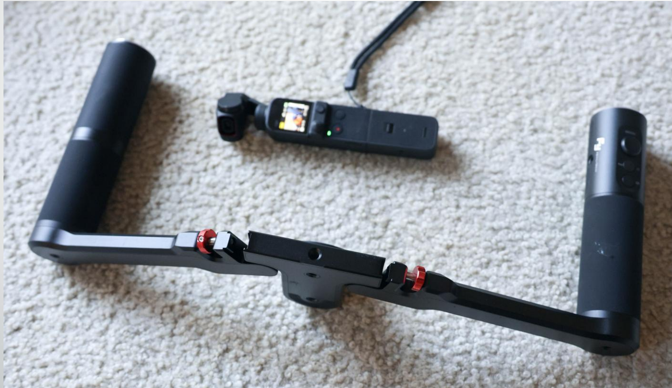
Blogging camera with built-in gimbal Handle for part of a 35mm-style camera gimbal
